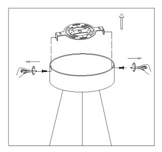
Step 1: Separate the bracket and fixture.
