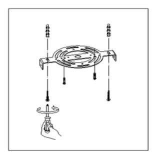
Step 2: Fix the bracket on the ceiling
