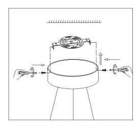
Step 4: Install the fixture on the bracket
