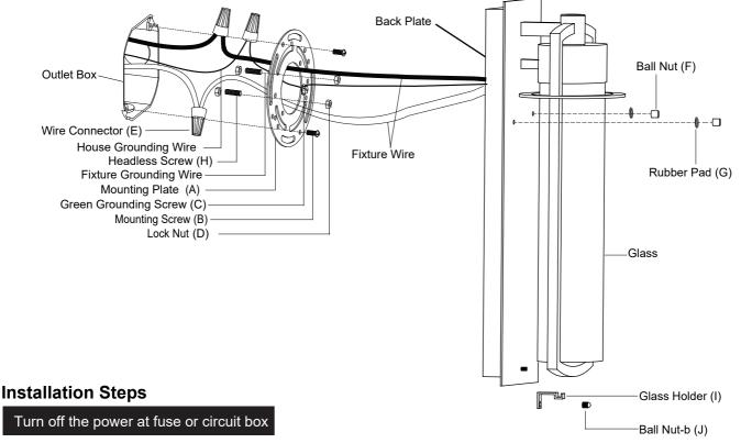
Thread two headless screws (H) through the mounting plate (A), then secure them with four lock nuts (D) ( two on each side of the mounting plate (A) ). Adjust the length of the headless screws (H) if necessary ).
